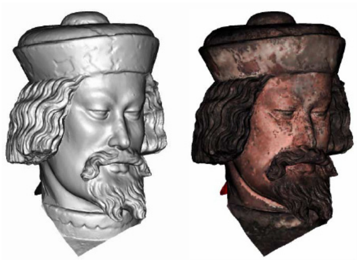
Fig. 6: Visualization of a St. George statue from the Germanic National Museum, Nuremberg. Left: Only geometry, without texture. Right: With reconstructed texture.
