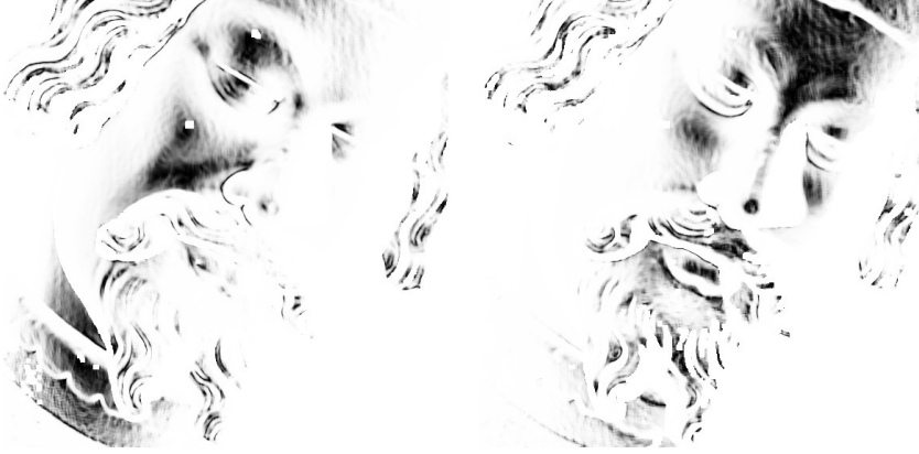
Fig. 2: Examples of confidence masks for influence of specular reflection. Left: illumination from left. Right: illumination from right. Note that the highlights (black regions, i.e. low confidence values) are in non-overlapping areas.
